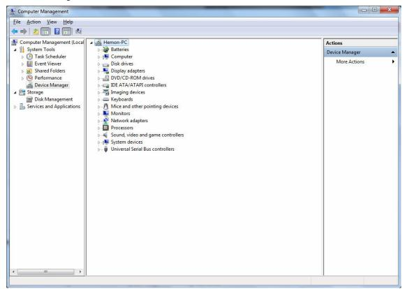
2) The USB driver is only active when the ACEECA device is trying to communicate with the PC. Hence you may have to try a USB Hotsync again to see the 'Device Manager' window below. You may have to open the 'Other devices' category by clicking on the little triangle icon to see the 'Meazura' device.
